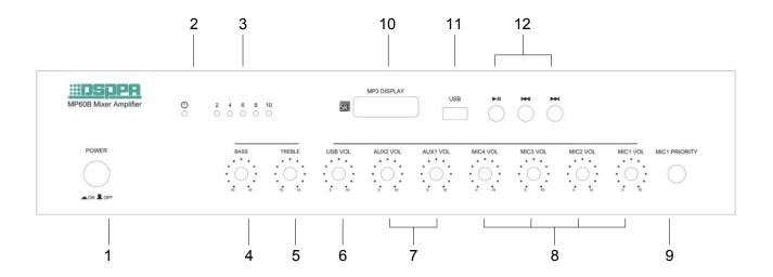
1. Power switch(power indicator lighting as ON state)
